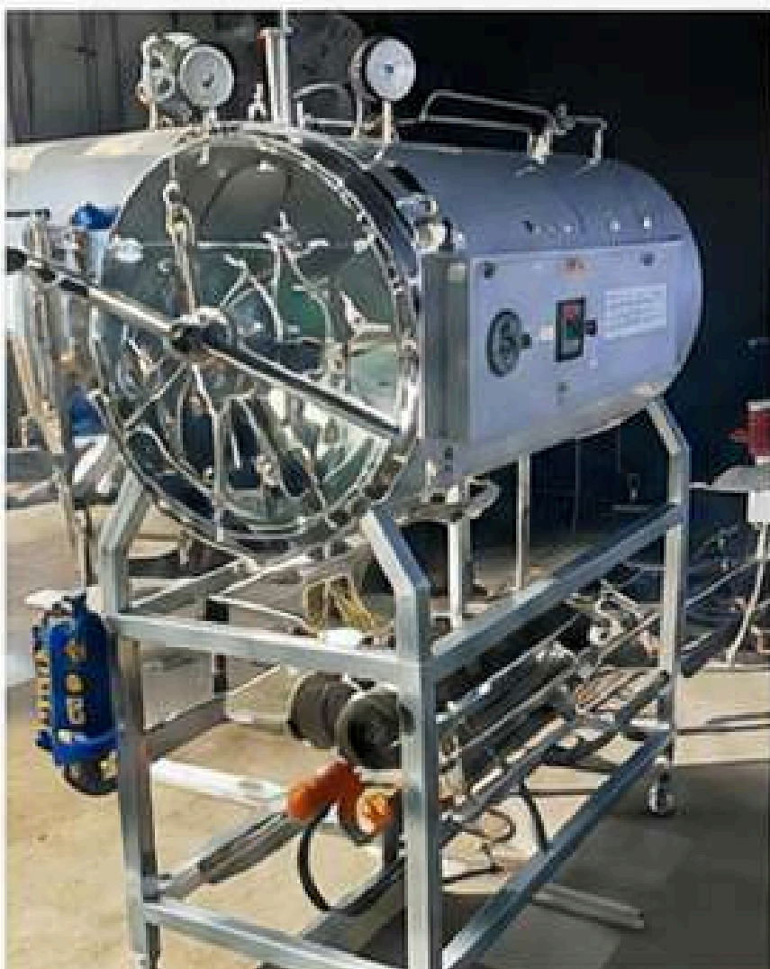
36-LTRS HORIZONTAL CYLINDRICAL AUTOCLAVE
